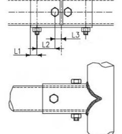
The removable connections type 1 (left) and 2 (left under & under) must be used for joining the upper parts of the main rollbar, the front rollbar and the lateral half-rollbars together.
