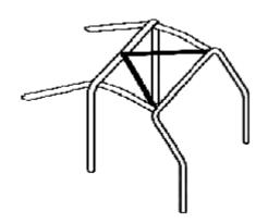
Tube which runs longitudinal from one of the highest points of the B-bar to the other side of the A-bar, must also be reinforced in each corner according to the drawing beside.
