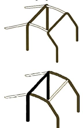
Two lateral rollbars two transversal members two backstays six mounting feet With this construction the diagonal member must be made double as a cross, right behind the seats.
