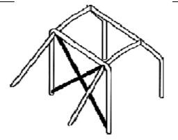
Diagonal member may also be designed as an inverted V, but then must also the roof reinforcement be shaped like a V.
